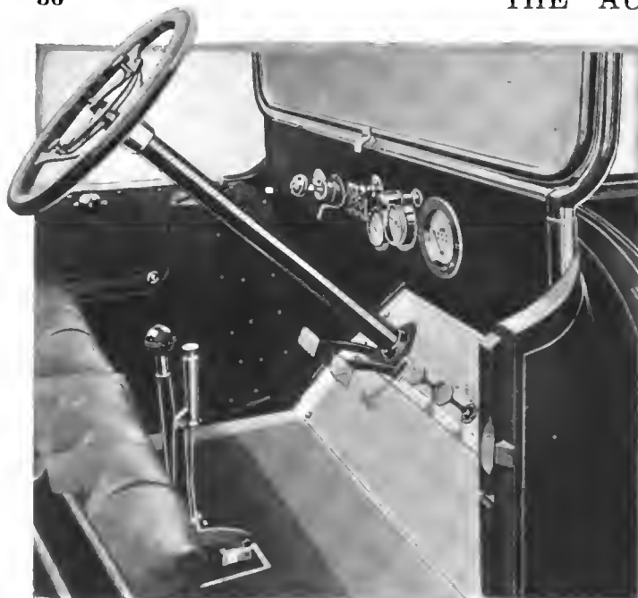
Control features of 1915 Chandler, showing left drive and center control as well as the arrangement of instruments on the cowl dash
